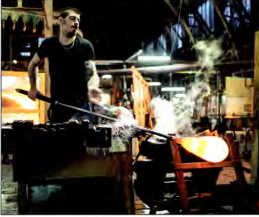
FIG. 2: The starter shapes the glass taken from the furnace.
