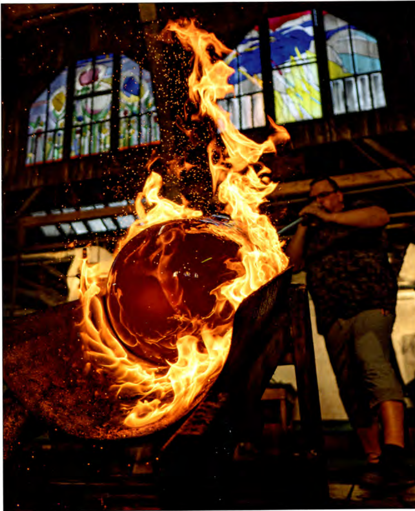
FIG. 3: One of Lamberts' master glass blowers inflating the balloon.
